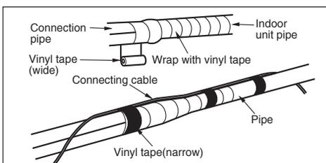
3. Bundle the piping and drain hose together by wrapping them with vinyl tape over the range within which they fit into the rear piping housing section.
