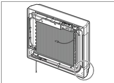
2. Assemble connecting lead wire with controller, fix the upper part of panel front, and match the lower part of panel front.
