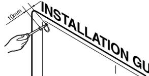
8. Drive the lower parts after facing the hole of product with plastic anchors, and fix completely the upper screws.
