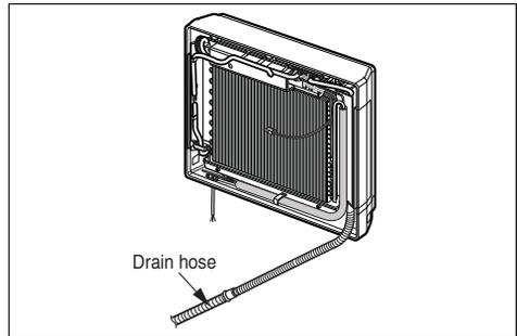
2. Tape the tubing, drain hose and the connecting cable. Be sure that the drain hose is located at the lowest side of the bundle. Locating at the upper side can cause drain pan to overflow inside the unit.
