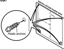
7. Hang the hole of product at the upper screws, and remove the map. (Falling attention)
